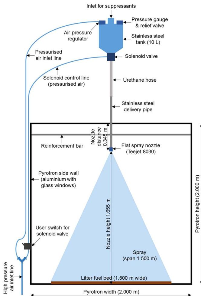
Fig. 1. Schematic diagram showing suppressant application system and cross section of Pyrotron working area viewed end-on (i.e. fire spread is out of the page).
