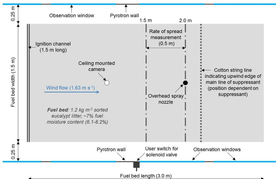
**Fig. 2.** Plan view of fuel bed and experimental setup in the CSIRO Pyrotron. Fire spread is from left to right.
