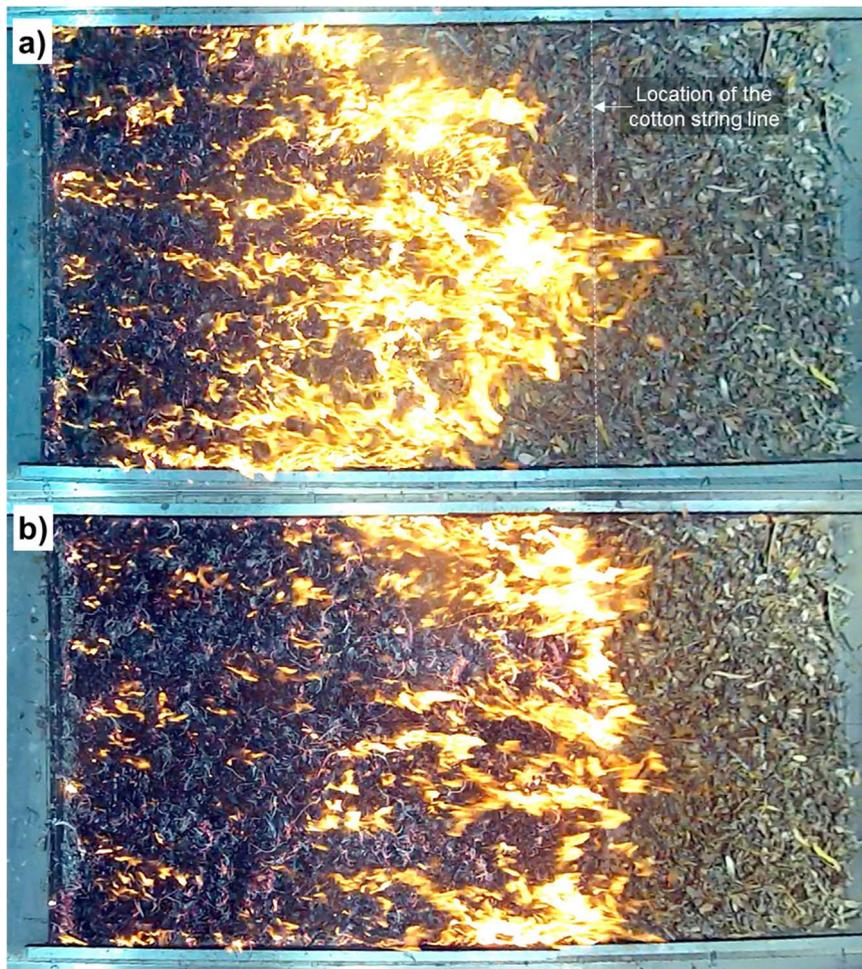
**Fig. 3.** Overhead view of suppressant evaluation test fires burning from left to right (a) immediately before suppression and (b) during suppression application. Note the change in the overall shape of the fire as suppression stops forward spread of the head.
